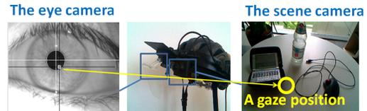
**Figure 1:** The SMI head-mounted eye tracker and sample views of both cameras.
