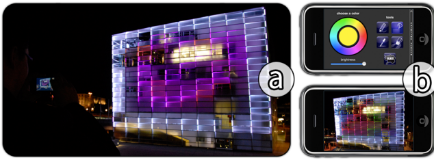
Figure 3. (a) Users can interact on the entire façade using their mobile device. (b) They choose their individual color and tool and apply these to the façade directly through live video [4].
