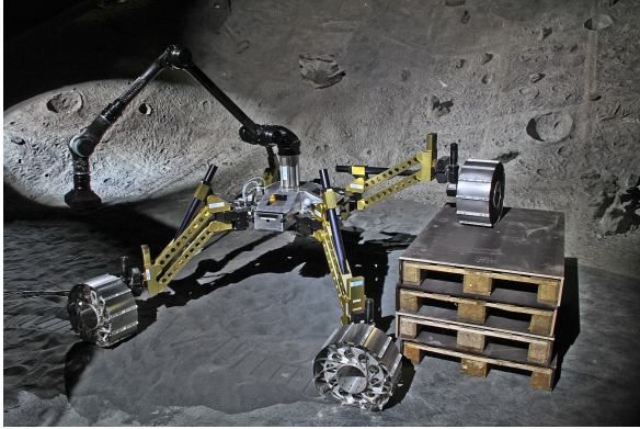
Figure 2. Current state of Sherpas integration study. In this picture the active suspension is used to step onto an obstacle. The arm is used to actively influence the center of gravity for improved stability.
