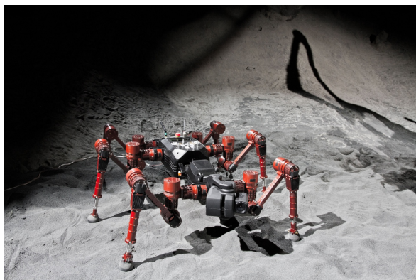
Figure 3. CREX robot in artificial crater environment. CREX is equipped with an electro-mechanical interface for attaching to Sherpa and for carrying payload-items.
