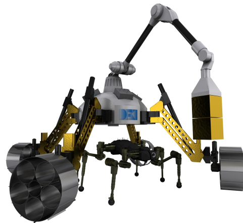
Figure 1. Parts of the RIMRES-System: Hybrid wheeled-leg rover Sherpa, legged scout CREX and immobile payload-items for building infrastructure and expanding the capabilities of the mobile systems.
