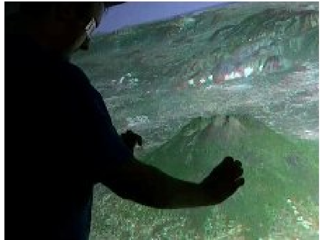
Figure 1: Interaction with stereoscopic projected geographic data on a multi-touch wall with anaglyph display.
