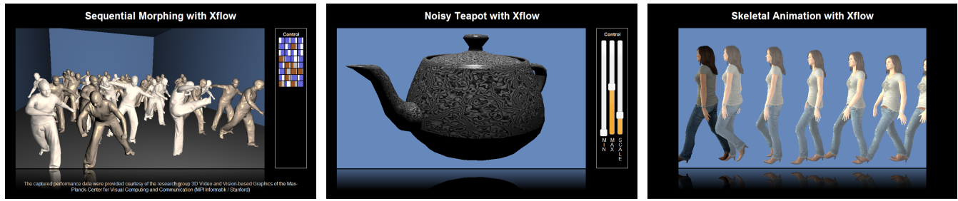
Figure 1: 3 example applications with Xflow. Each screen shot shows a web page that uses XML3D and Xflow to render real-time 3D graphics with advanced data processing. The left picture uses multiple instances of mesh interpolation for animation. The middle picture shows a dynamically generated noise texture. The right screen demonstrates multiple instances of skeletal animations.
