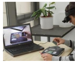
Figure 23 Example of online workflow assistance. The user wears an HMD with integrated camera. The task consists in changing the memory of a laptop. The right image shows what the user sees in the HMD while performing the task.
