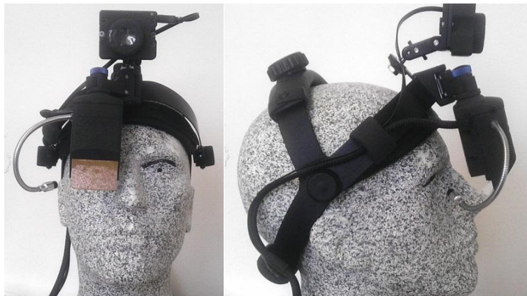
Figure 7 Monocular see-through HMD with integrated gaze tracking camera and attached Cam-IMU.
