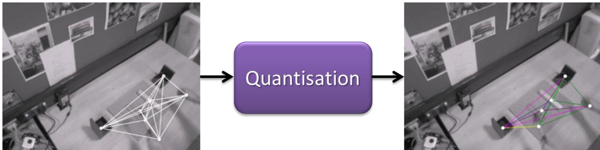
Figure 17 Quantisation of pairwise spatiotemporal relationships between key objects in the workspace.
