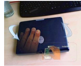
Figure 23 Example of online workflow assistance. The user wears an HMD with integrated camera. The task consists in changing the memory of a laptop. The right image shows what the user sees in the HMD while performing the task.
