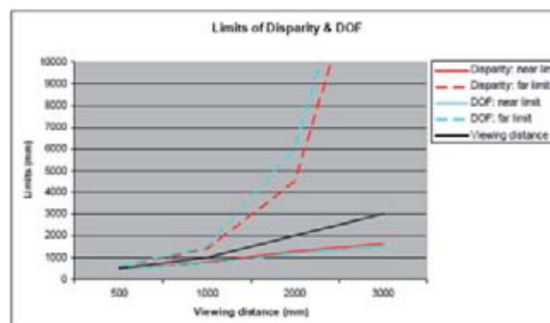
Abbildung 7: Limits of depth of focus (DOF) and binocular disparity for different viewing distances (Lambooj 2007).
