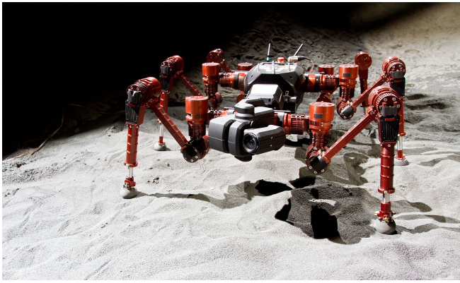
Fig. 2. The six-legged walking robot CREX which acts as scout in the aspired mission scenario of RIMRES.
