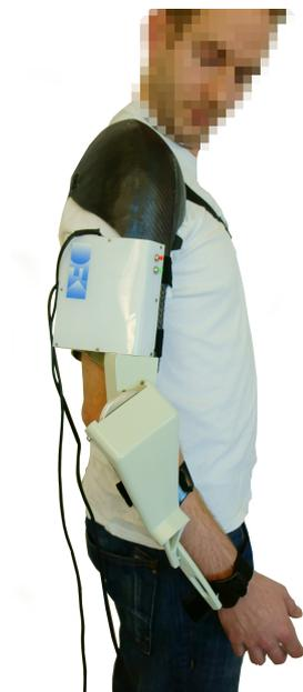
Figure 4: Design of the active orthosis.
