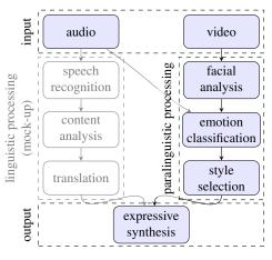
Figure 1. System architecture of FEAST
