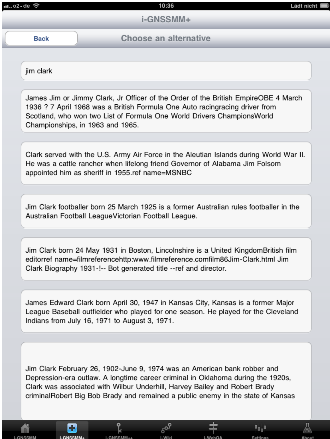
Figure 6.2: The disambiguation unit presents the first sentences of the Wikipedia abstract for each possible instance. In most cases it contains a definition of the term in question. The user now can choose one of the instances by simply touching it. The first entry can be chosen if no desambiguation is desired.
