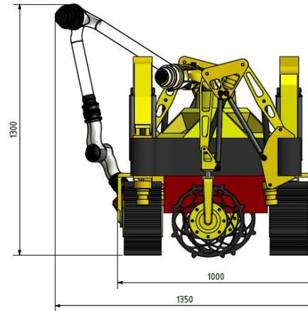
**Figure 8.** New stow pose of Sherpa. Note that the manipulator is unchanged in this design and might be adapted in a later development stage. Indicated dimensions are in mm.
