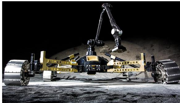
**Figure 1.** Sherpa in low stance mode. The body is very close to the ground and a wide footprint is adopted.
