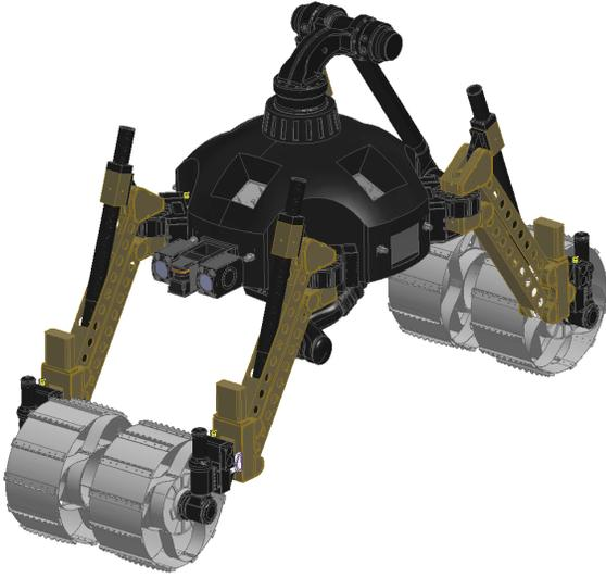
**Figure 4.** Sherpa in its minimal volume configuration. Due to the clustering of four out of six actuators at the end of each leg, more compact configurations are not possible.
