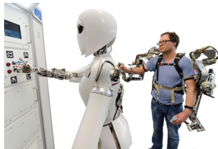
Teleoperation of the RIC humanoid robot AILA.
