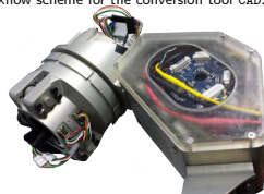
An integrated actuator at the shoulder.
