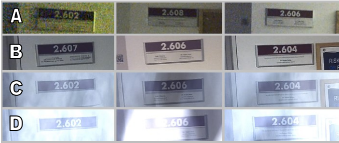
Figure 5. Door plates in various conditions. Row A is in darkness. Row B is in light. Row C is in smoke and Row D is in heavy smoke. Note that camera exposure automatically adjusted for lighting conditions.
