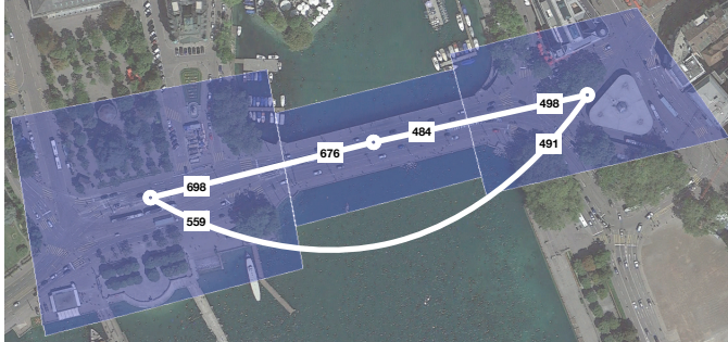
Fig. 9. Diagram showing Bluetooth re-discoveries on the Quai Bridge. The numbers towards the end of a line section represent the number of Bluetooth devices re-appearing afterwards at the target zone. The blue colored regions represent the detection area.
