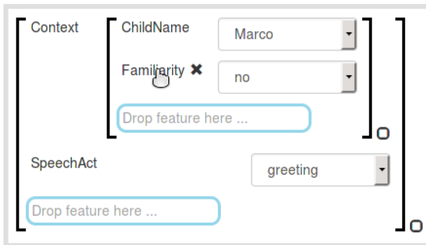
Figure 13: Visual representation of an LHS. The mouse cursor points to the name of a feature ( Familiarity ) belonging to a nested AVM. As a result, the system shows a button for removing this feature, as well as two buttons for emptying the nested and top-level AVMs.
