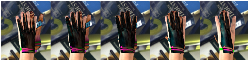
Figure 5.21: Difference images between (synthetic) observation and our rendering |I^{obs} - I_\alpha^{render}| for several values of \alpha . The center image shows \alpha = 0.5 , where the ground truth optimum is located. The objective function for 0 \leq \alpha \leq 1 was evaluated in 2000 randomized repetitions in both experimental setups (clutter setup shown here).
