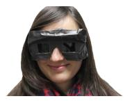
Figure 4: Our prototype consisting of modified ELSA 3D Relevator glasses. Top: Open shades, the user is anxious Bottom: closed glasses, the user is facing danger more relaxed. rate monitor that detects the increase of stress and arousal, the glasses can be set to black out the vision and leave the user with only the sound. Thus relaxing his mind by not having to watch a disturbing or frightening scene.
