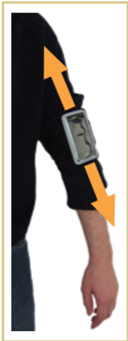
Figure 2. An example of “within body part” displacement. The placement of the device, although located on the arm, can shift up or down.
