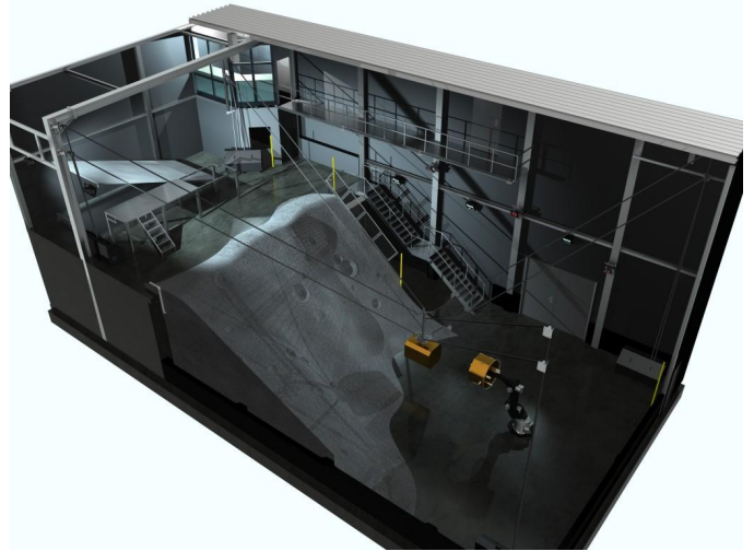
Figure 3: Overview of the Space Exploration Hall. One can identify the cable robot and the robotic arm which carry the satellite mock-ups. The control room on the upper left corner provides a good overview of the facility. A balcony has been added to be able to monitor the systems from above, with no risk of entering into the working areas of the robotic systems.
