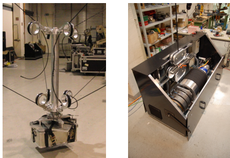
(a) First test of the mount with eight cables attached in two virtual points (b) A winch for winding two cables simultaneously
