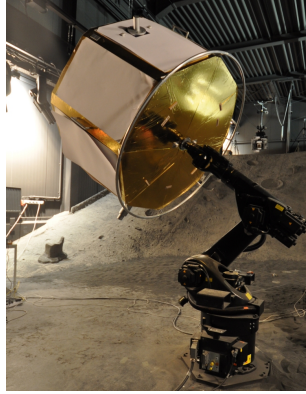
(b) A 6-DOF robotic arm is used to move the Client satellite
