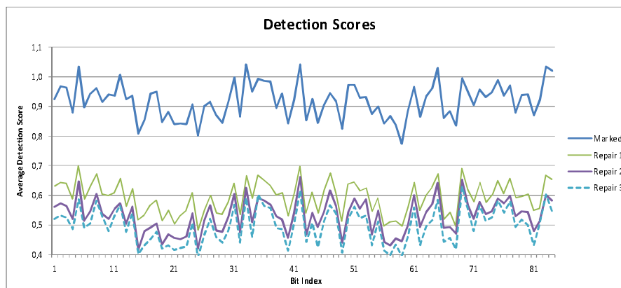
Figure 6: Detection scores of the 84 message bits; upper curve: score from marked audio (no stretching attack); lower three curves: score after 1, 2 and 3 recursive stages of repairing
