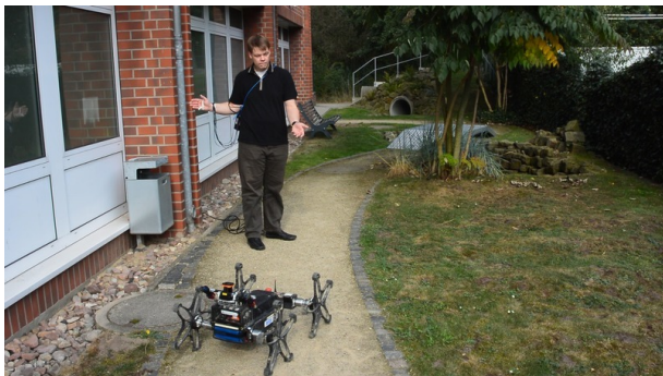
Figure 10. Image of first outdoor tests; the rover is controlled by (simplified) gesture commands - basically, after being set into a “attention” mode, the rover mimics the movements of the user’s arm [e.g. it moves forward, if the arm is moved into that direction, or starts to rotate if the arm is moved sideways]
