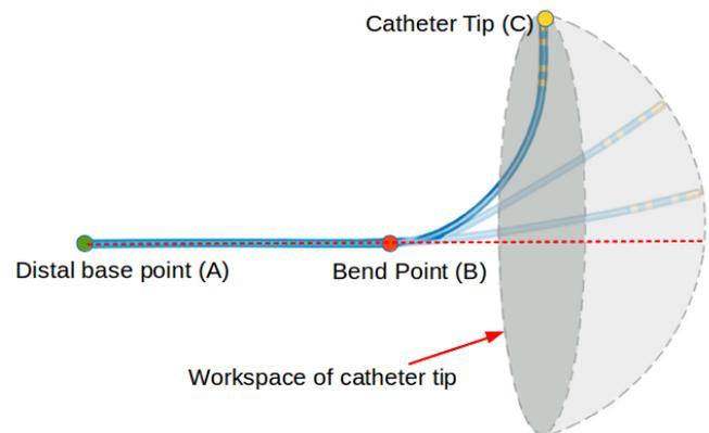
Fig. 2. The catheter steering mechanism and the corresponding bowl shaped catheter tip workspace.
