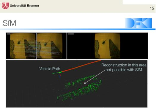
Sparse pointcloud generated by Structure from Motion
