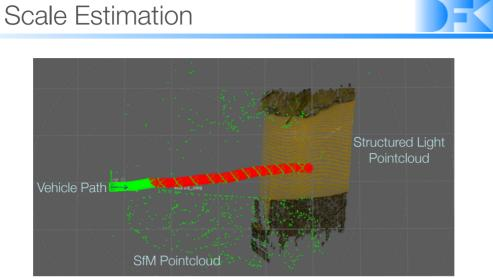
For each key frame ~10-20 features are used to fix the scale
