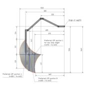
Range of motion of one leg in cut view (mock-up leg for dimensions is shown).
