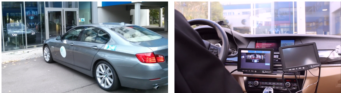
Figure 9.12 – The demonstrator setup. The urban display is simulated by a billboard inside the DFKI building. Two touch screens are mounted at the cockpit of the car.
