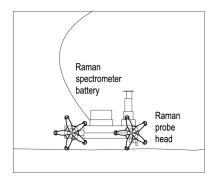
rover outfitted with Raman specrometer in payload box and probe head at front bottom
