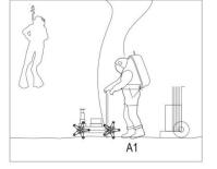
rover functions as support for the first upright beam to be held in position
