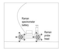
rover outfitted with Raman specrometer in payload box and probe head at front bottom
