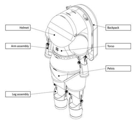
Figure 6. Design of the exoskeleton of the EVA training suit. The exoskeleton will be covered by an oversuit, not shown; *Credit: MOONWALK consortium, visualization: Comex, 2015.*
