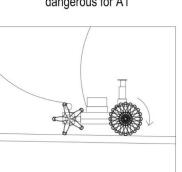
rover front wheels start spinning while the rear wheels are locked
