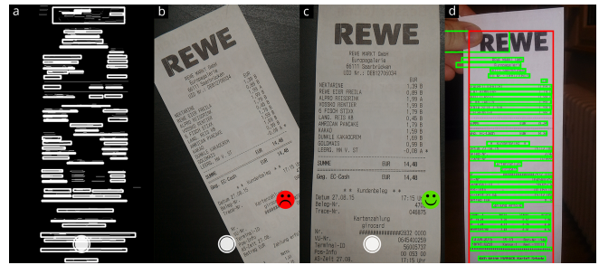
Figure 5: a) Identified horizontally aligned regions, b) Unfavorable position of the camera, c) Suitable picture, d) Region Of Interest (ROI)
