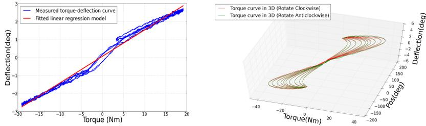
Fig. 6. Torque-spring deflection curves with 10 different load positions. *left*: A fitted linear regression model (red line):  $\tau = a * \theta_s + b$  is used for representing the measured torque-spring deflection curve (blue line), where  $\tau$  is the motor torque and  $\theta_s$  is the deflection of the spring. *right*: The motor rotating position is used as the third dimension for training the DGMM model.
