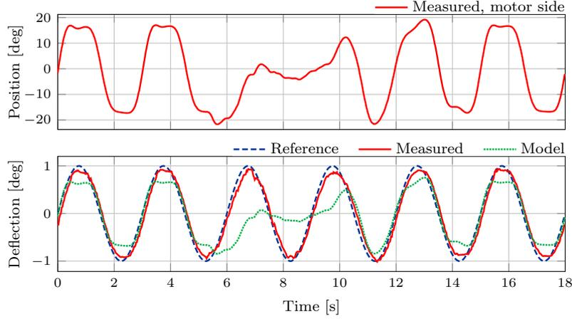
Fig. 5. Result of deflection control acting against an external disturbance. The top figure shows the position 'before' the spring (motor side). The bottom figure shows the deflection measured using the difference of position between the sensors placed before and after the spring. In red, the deflection measured; in blue, the reference deflection  $x * \sin(\omega t)$ ; in green, the deflection according to the load torque, assuming a linear relationship
