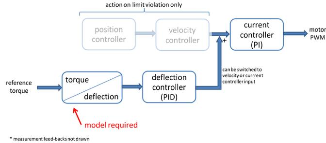
Fig. 4. Controller structure
