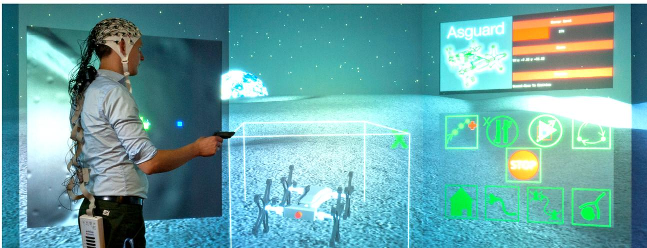
**Figure 1.** Immersive virtual 3D multi-robot control using a CAVE supported by embedded Brain Reading (eBR).
