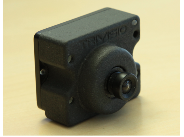
Figure 3: The inertial sensor with camera system used in this work.
