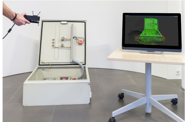
Figure 1: We present our new AR discrepancy check, which is able to capture scene geometry in real-time using an RGB-D camera. Discrepancies are detected while capturing with our new semi-automatic alignment and distance computation.
