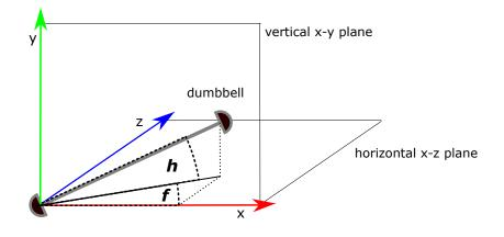
Figure 4.3: Sketch of the measured *height angle* (*h*) and *forward angle* (*f*).
