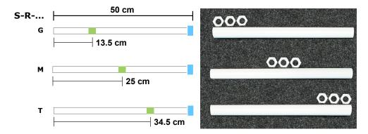
Figure 3.9: The concept drawings on the left show the **Stick Proxy** objects with the corresponding CM locations (green) and the location of the tracking target (blue). The notation **S-R-...** encodes the **S**tick's **R**eal shift to the **G**rip, **M**id location or the Top. The picture on the right shows the two real proxies with the inserted steel weights. The bottommost object is the topmost proxy after turning it around.
