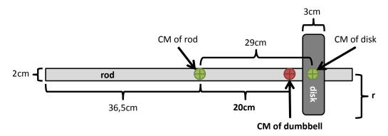
Figure A.1: Sketch of the rod and the disk that make up the virtual dumbbell with the CM shifted by 20*cm* to the right. The sketch is not true to scale.
