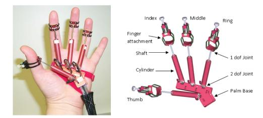
Figure 2.5: General appearance of a *Rutgers Master II - New Design* haptic interface prototype (left) and corresponding CAD model with sensors and actuators (right) © Rutgers University - Reprinted by permission. [31]
