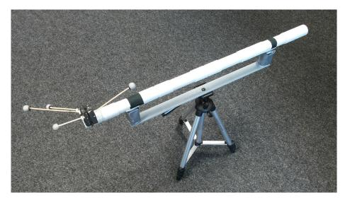
Figure 3.4: Picture of a balanced **Dumbbell Proxy** on the custom-built proxy stand.
