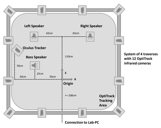
Figure 3.5: Sketch of the setup in the laboratory.
