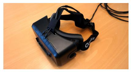
Figure 1.2: The *Oculus Rift DK 2* used in the experiments of this thesis. It is an example for a modern VR-HMD whose final version is going to be released for consumer markets soon.
