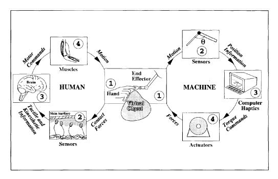
Figure 2.4: The Human and Machine Sensorimotor Loop [3]
