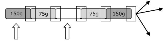
Figure 3.2: Sketch depicting the final proxy design concept. It illustrates the differently weighted chambers which are connected by union-connectors. The rigid body target is mounted on the right end and the two white arrows depict the grip- and center-grasp locations, respectively.
