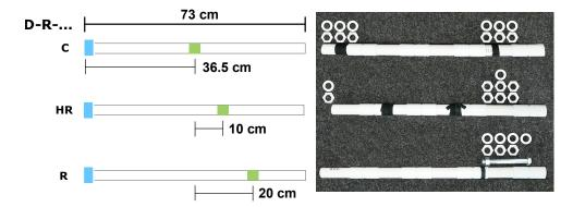
Figure 3.8: The concept drawings on the left show the **Dumbbell Proxy** objects with the corresponding CM locations (green) and the location of the tracking target (blue). The notation **D-R-...** encodes the **Dumbbell's Real shift** to the **Center**, **Half-Right** or **Right**. The picture on the right shows the real proxies with the inserted steel weights.
