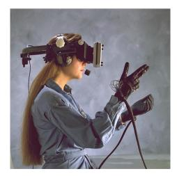
Figure 1.1: Picture of VR research at NASA during the 90s showing a VR-HMD and data gloves of that time [4]
