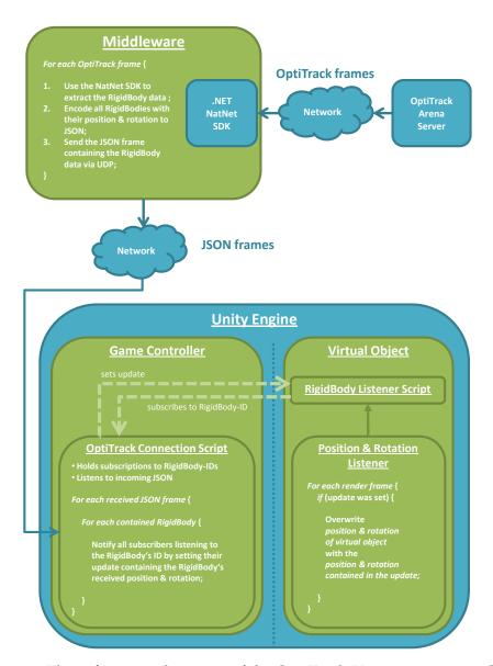
Figure 3.6: The software architecture of the OptiTrack-Unity integration. Green modules were developed and implemented for this thesis, blue modules indicate preexisting software.
