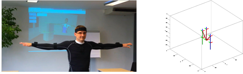
Fig. 3. (a) Sensor jacket with visualization in the background (b) Stick figure model of the upper body motion tracking with six segments
