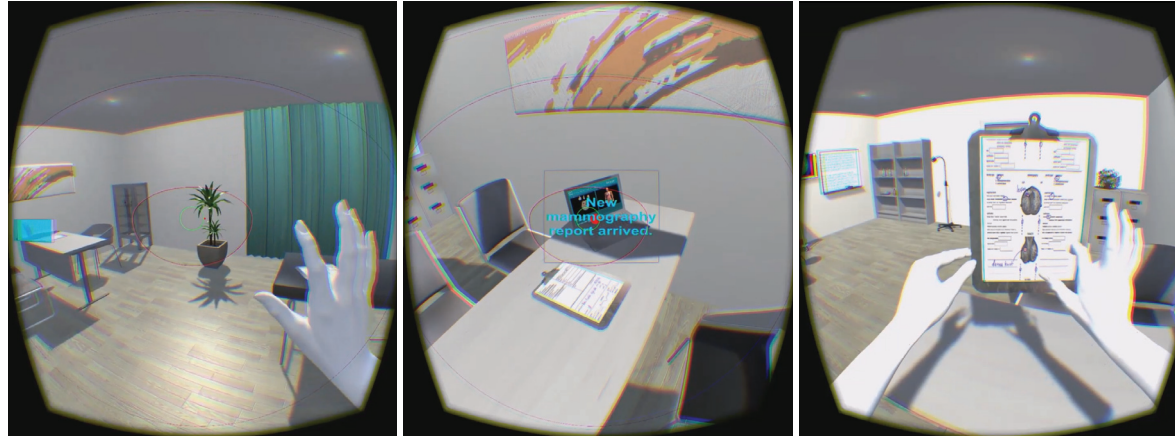
Figure 4: Our implemented medical use case. Left: In case a remote collaborator would like to share an EPR, the context-aware peripheral analysis component of our system informs the user by visual augmentations (blue highlighting). Middle: Based on the visibility of the object of interest to the user, more detailed information overlays are presented. Right: Interactive visualisation/exploration of annotated patient data. See demo video at https://www.dropbox.com/s/2bkmn8vzmtmrvl2/file167-1.mp4 .
