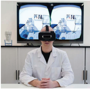
Figure 1: Our VR setup features an Oculus Rift DK2 HMD with SMI's integrated eye tracking component together with an attached Leap Motion controller for tracking hand movements.
