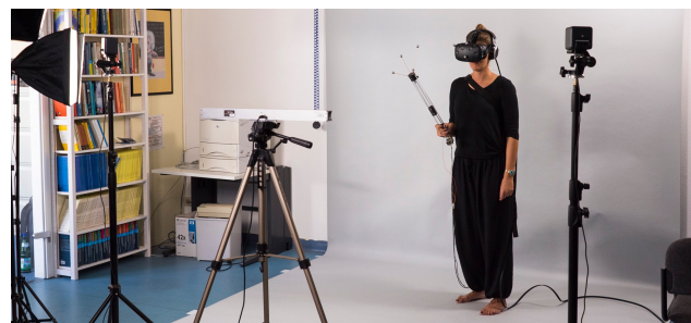
Fig. 5. A user interacting with Shifty in our experimental setup. The user wears the HTC Vive and headphones. The rigid-body target on the proxy is tracked by an OptiTrack system.
