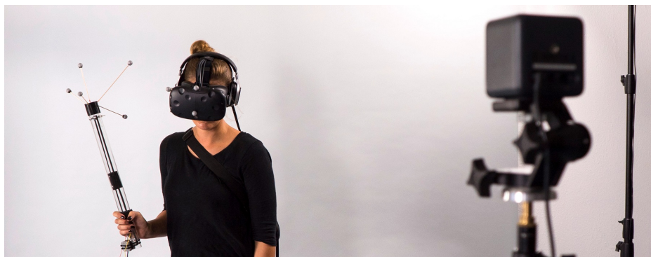
Fig. 1. A user interacting with Shifty in our experimental setup. Shifty is a rod-shaped dynamic passive haptic proxy that can change its internal weight distribution to automatically adapt its passive haptic feedback. Shifty can be used to enhance the perception of virtual objects and provides a compelling and dynamic passive haptic feedback.
