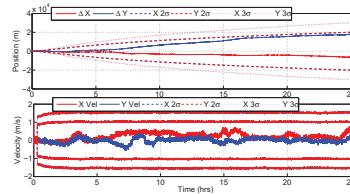
Sentry dive 298 with an IMU based prediction model. 19.7 km error after 25 hours with no DVL, with a 2.7km correction with DVL bottom-lock.
