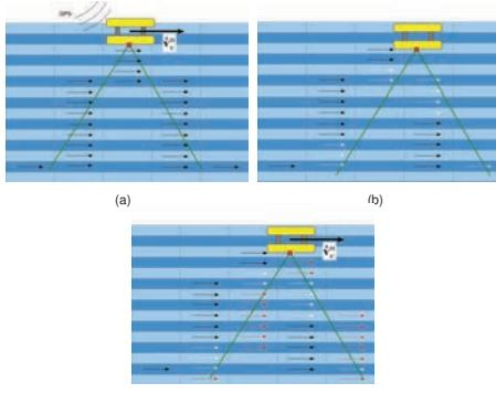
ADCP aiding method sequence in the mid-water (a) Initial GPS position and velocity are known, and water velocities with black arrows can be deduced. (b) The AUV moves, and repeatedly observes the same current bins, shown as white arrows. (c) The AUV velocity in the world frame can be deduced, along with new current bins shown in red.
