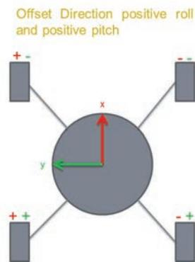
Fig: Offset directions for positive roll and pitch errors
