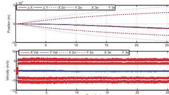
Sentry dive 299 with a constant velocity based prediction model. 17.3 km error after 25 hours with no DVL, with a 1.5 km correction with DVL bottom-lock.
