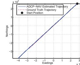
The estimation result is compared to the ground truth from USBL for Sentry 299.
