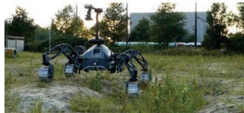
Photograph of SherpaTT while driving through a sand pit, keeping the roll/pitch deviation of the body at a minimum
