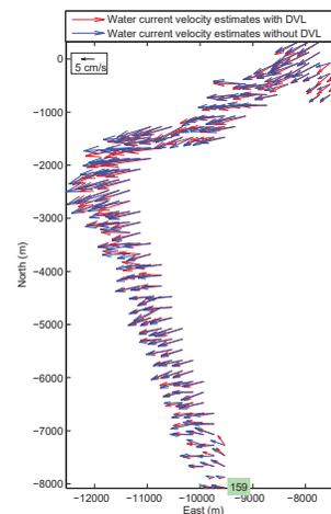
Water current velocity estimates with and without DVL with differences for the North and East velocity estimates within 2 cm/s. The processing time for the 10000 second mission in MATLAB on an Intel i7-4770K CPU at 3.50GHz was 3672 and 3016 seconds with and without DVL respectively, indicating real-time feasibility.
