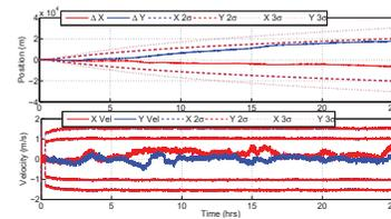
Sentry dive 298 with an IMU based prediction model. 19.7 km error after 25 hours with no DVL, with a 2.7km km correction with DVL bottom-lock.
