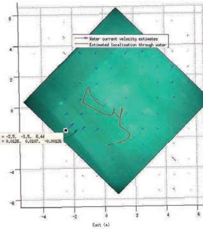
The hose is seen in the bottom left of the figure. The water current signal appears from that region. The reported accuracies by the filter were about 6 mm/s ( $2\sigma$ ) for the water currents where the water current signal of approximately 1.5 cm/s. The water current estimates were calculated in MATLAB, with a processing time of 527 seconds, thus showing potential real-time application.
