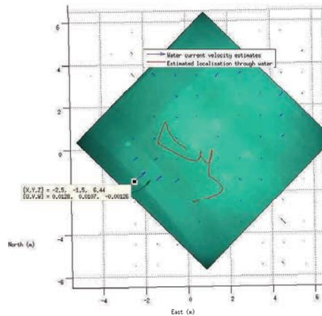
The hose is seen in the bottom left of the figure. The water current signal appears from that region. The reported accuracies by the filter were about 6 mm/s ( $2\sigma$ ) for the water currents where the water current signal of approximately 1.5 cm/s. The water current estimates were calculated in MATLAB, with a processing time of 527 seconds, thus showing potential real-time application.
