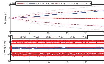
Sentry dive 298 with a constant velocity based prediction model. 27.5 km error after 25 hours with no DVL, with a 1.5 km correction with DVL bottom-lock.
