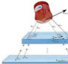
The ADCP sensor possesses 4 beams in a Janus configuration, 30 degrees from the vertical. This allows fore, aft, port and starboard direction sensing capability.
