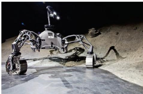
Photograph of SherpaTT equipped with flexible wheels and manipulation arm
