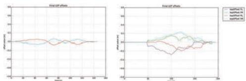
Plots of LEP-offsets. Left: for pure FLC (same Offset for pairs FL/RR and FR/RL). Right: FLC+RPA generate different offsets for all LEPs to keep the robot level with the ground
