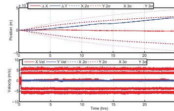
Sentry dive 298 with a constant velocity based prediction model. 27.5 km error after 25 hours with no DVL, with a 1.5 km correction with DVL bottom-lock.
