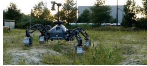
Photograph of SherpaTT while driving through a sand pitch, keeping the roll/pitch deviation of the body at a minimum.
