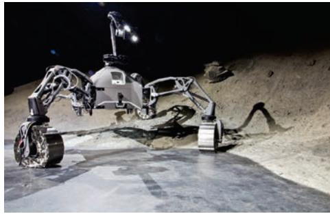
Photograph of SherpaTT equipped with flexible wheels and manipulation arm
