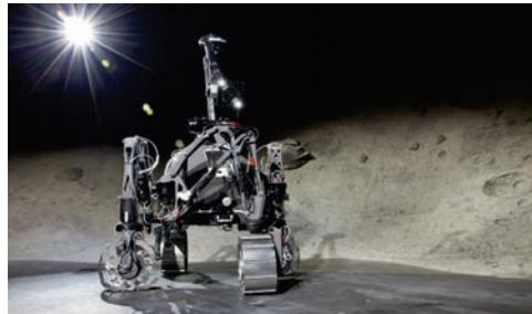
Photograph of SherpaTT with its legs in stow configuration
