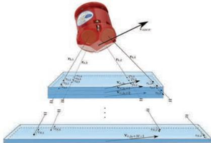
The ADCP sensor possesses 4 beams in a Janus configuration, 30 degrees from the vertical. This allows fore, aft, port and starboard direction sensing capability.
