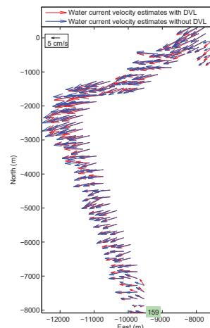
Water current velocity estimates with and without DVL with differences for the North and East velocity estimates within 2 cm/s. The processing time for the 10000 second mission in MATLAB on an Intel i7-4770 CPU at 3.5GHz was 3672 and 3016 seconds with and without DVL respectively, indicating real-time feasibility.
