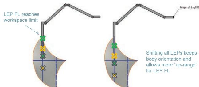
Fig: Example for simple LEP-Shifting for workspace optimization
