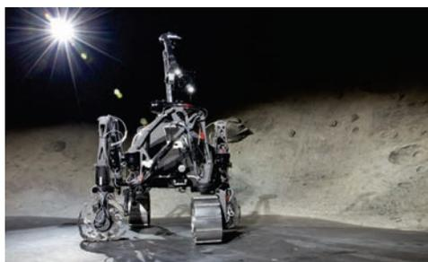
Photograph of SherpaTT with its legs in stow configuration
