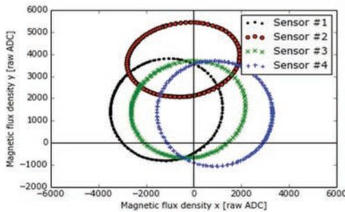
Magnetometer Readings (xy-plane) during 360° turn – Crawler Wally
