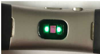
Figure 3: An optical heart rate sensor of a Microsoft Band 2 with light emitting diodes.
