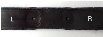
Figure 2: Chest strap of a Garmin Forerunner that measures heart rate with two electrodes that acquire an EKG signal.
