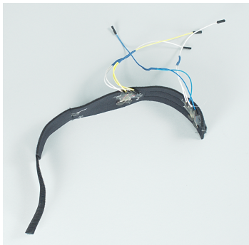
Figure 5: Vibration motors attached to an elastic strip to give real-time feedback while running.
