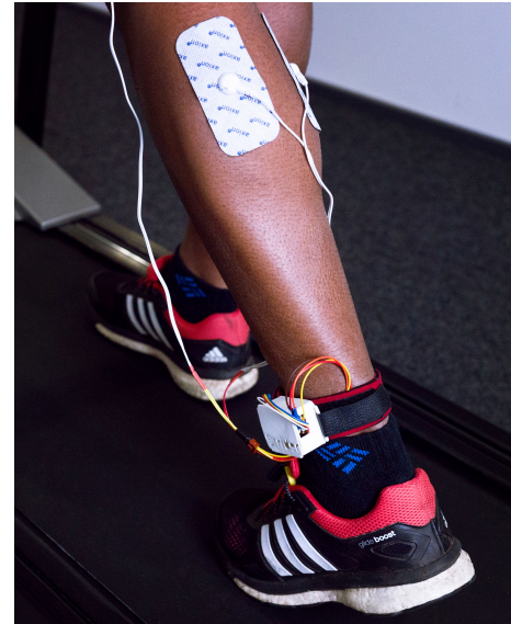
Fig. 4. Placement of the EMS electrodes and wearable control unit.
