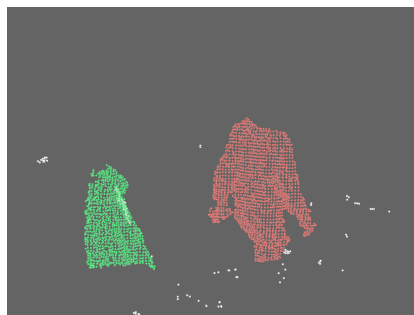
(c) after voxel grid filtering and clustering (red/green: the two object clusters; white: ignored clusters below the size threshold)
