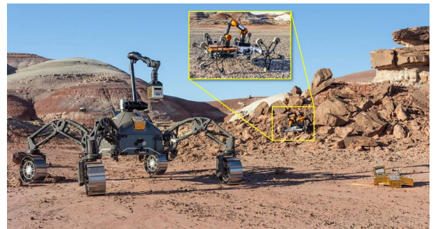
Figure 1. The employed systems in the field trials: Hybrid wheeled-leg rover SherpaTT (left, with modular sampling tool attached to the manipulator arm), Coyote III (center background and inset, with modular manipulator arm SIMA) and BaseCamp (right, with attached sample container)
