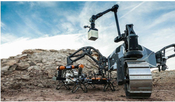
Figure 10. Rendezvous of SherpaTT and Coyote III during the mission sequence. Coyote III's manipulation arm SIMA is in a pose to give room for transfer of the sample container.
