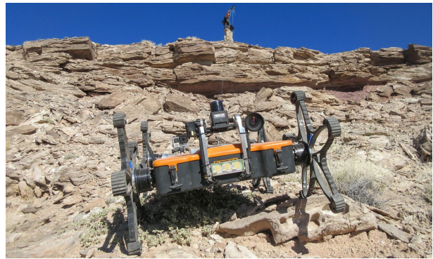
Figure 5. SherpaTT during a single system test concerning slope driving capabilities (top) and Coyote III in preparational tests for cliff exploration scenarios (bottom)
