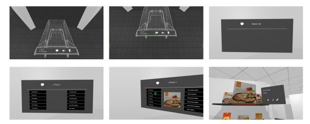
Fig. 8. **Speech input.** Here, the user starts by gazing at the speech button, and speaks the search term into the microphone. After the search results are displayed, the user can select the desired product in order to be moved to the desired shelf.
