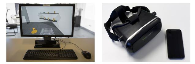
Fig. 9. This figures show the **output devices** we used for our prototype. On the left: 22 inch display with Microsoft Kinect 2 for speech input and a standard mouse for camera control. On the right: a common smart-phone VR case and LG Nexus 5X.
