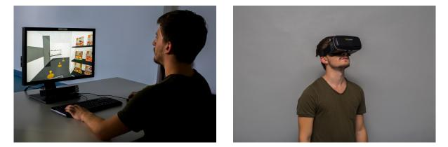
Fig. 10. Left: **Desktop setting.** Here, the participant controls the camera by moving the mouse with her/his dominant hand. The speech was recorded by a Microsoft Kinect 2, placed under the display. The keyboard shown in this picture had no effect and was not used in the experiment. Right: **VR setting.** Here, the user controls the camera by moving her/his head. Speech was recorded by the smart-phone's microphone.
