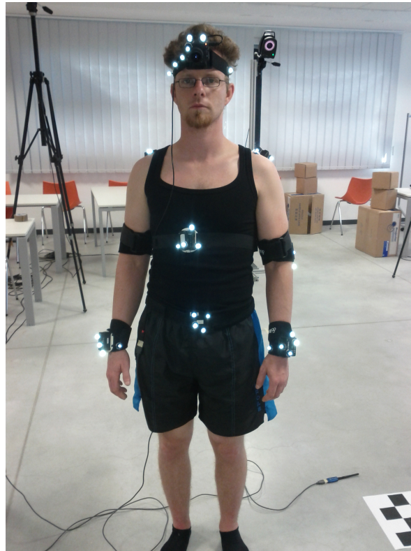
Figure 5. Experimental setup showing markers that were placed on the anatomical landmarks and on the 9 mIMUs.
