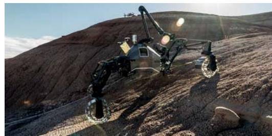
Fig. 9. SherpaTT during field trials in Utah, USA in Oct/Nov 2016. Slope in this image is about 28°/53% and covered with duricrust. SherpaTT uses FLC and RPA modules to climb the slope.
