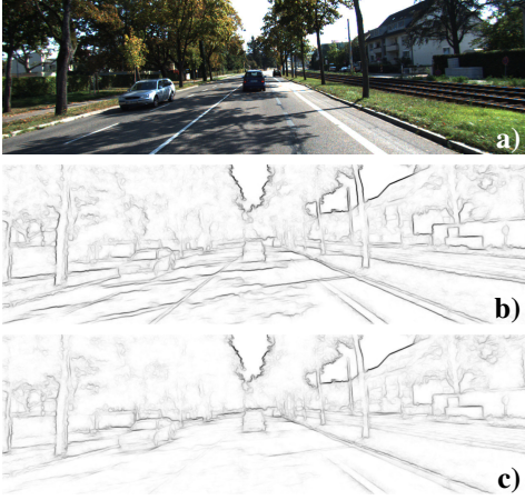
Figure 4. Whereas SED [8] (b) detects all image boundaries, our new boundary detector (c) suppresses lane markings and shadows.
