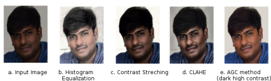
Figure 2: various contrast enhancing techniques. Over or under-enhancement in b,c,d. We use AGC (Rahman et al., 2016) in our approach
