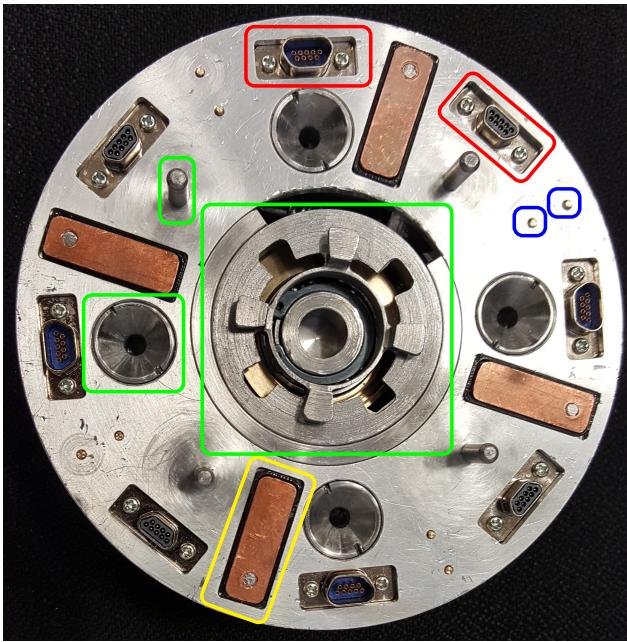
**Figure 3. Prototype of the standard interface. Green, red, blue and yellow boxes indicate the mechanical, data, power and thermal functionalities, respectively [26].**
