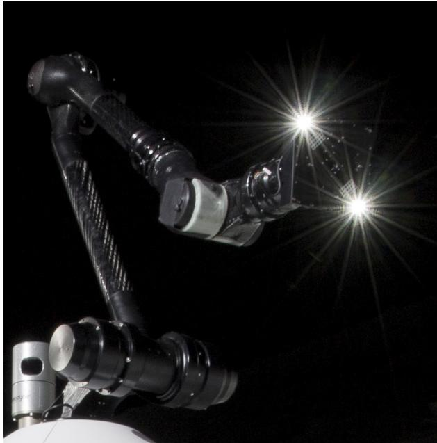
**Figure 7. End-effector of SherpaTT rover (credit: DFKI 2015).**
