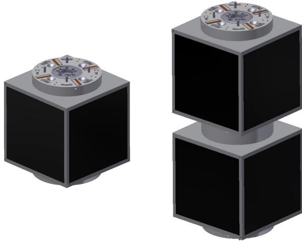
**Figure 4. CAD models of an APM housing with external interfaces in single and stack configurations, respectively.**
