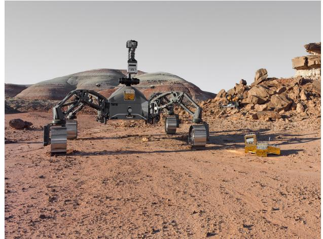
**Figure 2.** Real world test of a multi-robot planetary exploration scenario using modular payload-items (PLIs) performed by DFKI at the Utah desert USA. The main rover is visible in the center, PLIs on the right and an agile robot in the upper-right of the figure (credit: DFKI 2016).
