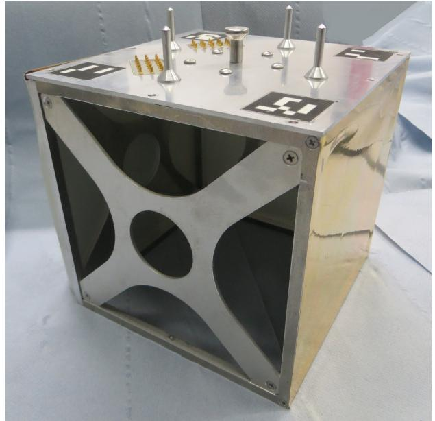
**Figure 6. Skeleton of a payload-item developed at DFKI [12].**
