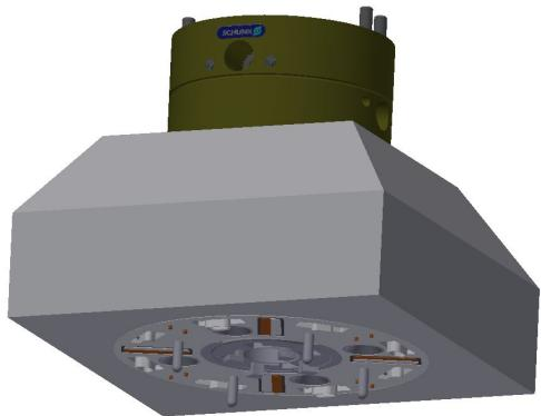
**Figure 11. CAD model of the reference concept of the end-effector.**
