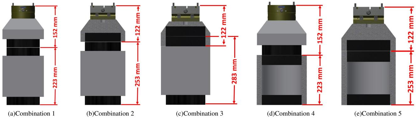
**Figure 10. Feasible EE-APM combinations considering three EE and two APM configurations.**
