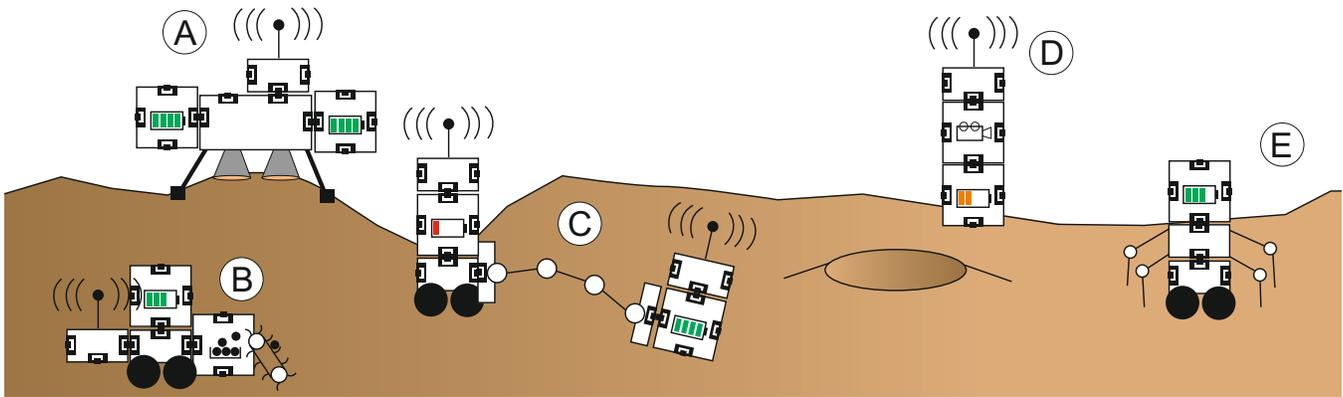
**Figure 1.** Schematic overview: A heterogenous robotic team with modular components in a Mars exploration scenario. Depending on the functionality, the payload-items serve as range extenders or allow the different systems to be equipped with different scientific modules, based on the context of the current mission.
