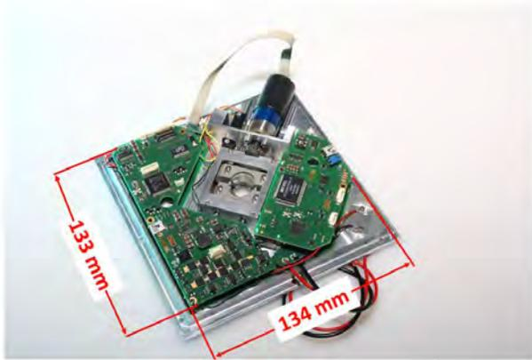
**Figure 12.** The three PCBs attached on the active part of EMI
