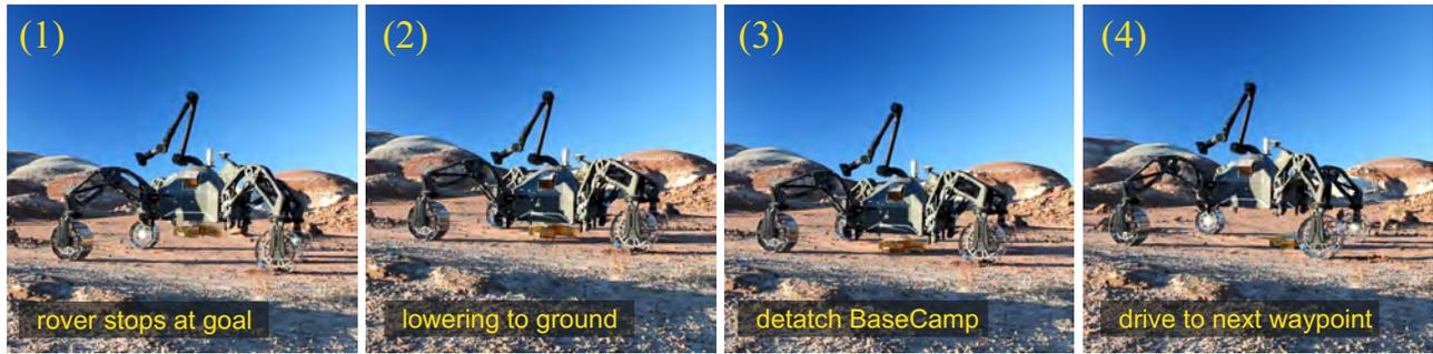
**Figure 17.** Sequence of BaseCamp deployment. From left to right: (1) SherpaTT stops driving and starts lowering of the body. (2) BaseCamp is close to the ground, feet are released. (3) Rover released BaseCamp and starts to move body upwards. (4) Driving away from deployed BaseCamp.
