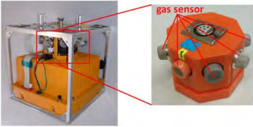
**Figure 7.** Gas sensor module
