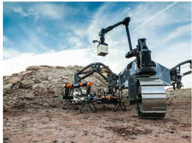
**Figure 18.** Part of the scenario of a logistics chain: SherpaTT is about to put the sampling module onto Coyote III.
