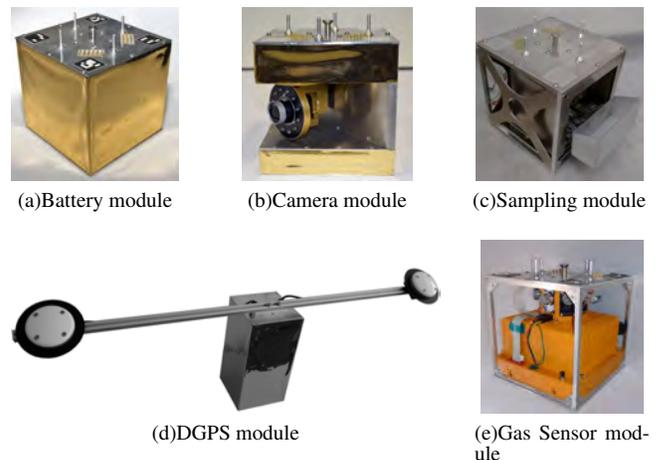
**Figure 2.** The five developed functional PLIs
