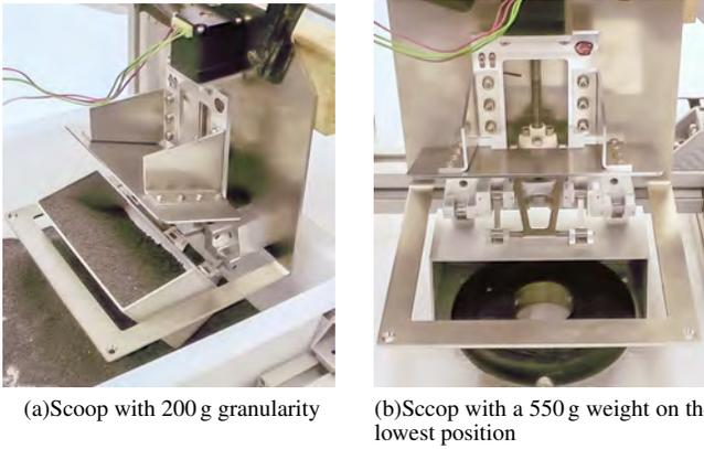
**Figure 14.** Weight tests with the scoop assembly
