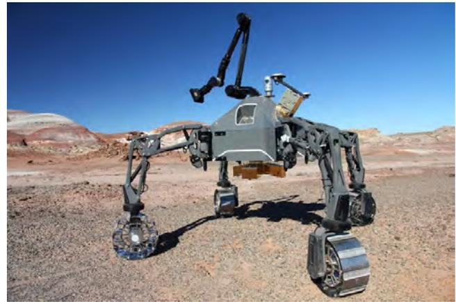
**Figure 6.** SherpaTT with docked BaseCamp to its body and DGPS module mounted to the rear payload bay. Rover is in its max body-ground clearance position.
