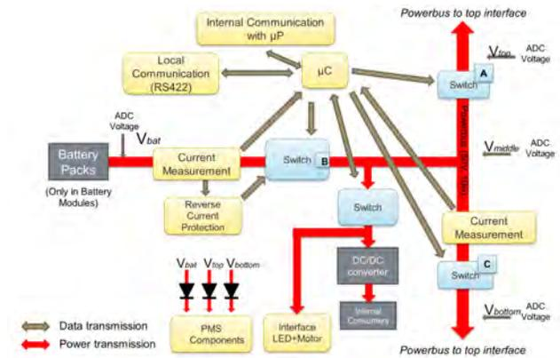
**Figure 13.** Hardware architecture of the PMS in individual PLIs
