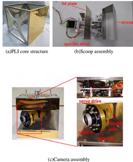
**Figure 4.** PLI core structure and assemblies of the sampling and camera module
