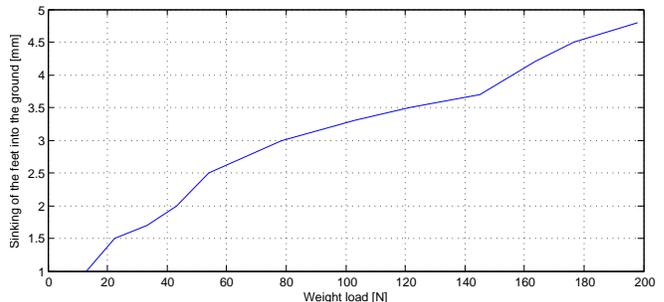
**Figure 16.** Weight tests with one foot of the BaseCamp
