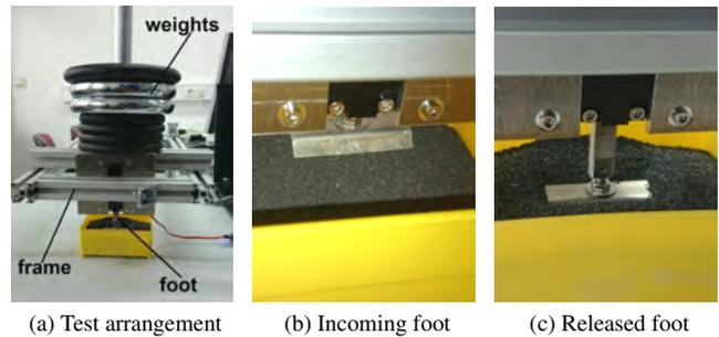
**Figure 15.** Testing the weight load capacity of the BaseCamp's feet
