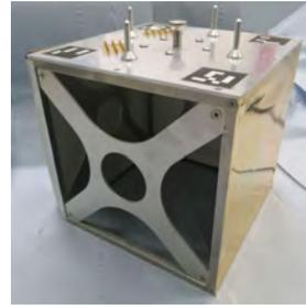
(a) Basic PLI with passive EMI on top, golden covering and cross-shaped stiffening
