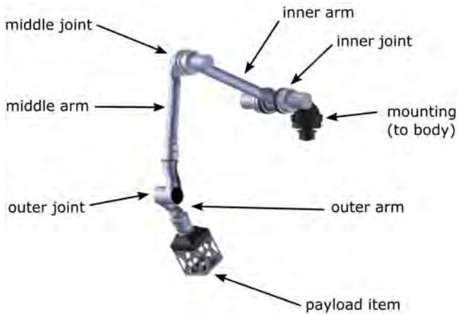
**Figure 5.** Schematics of SherpaTT's manipulator with mounted PLI.
