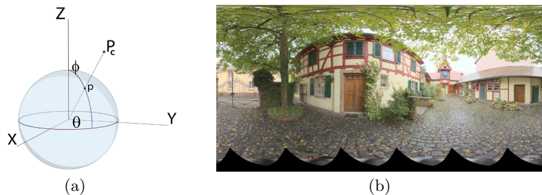
Fig. 1. (a) Spherical coordinates and illustration of the spherical projection. (b) Pixel-map of a spherical image.
