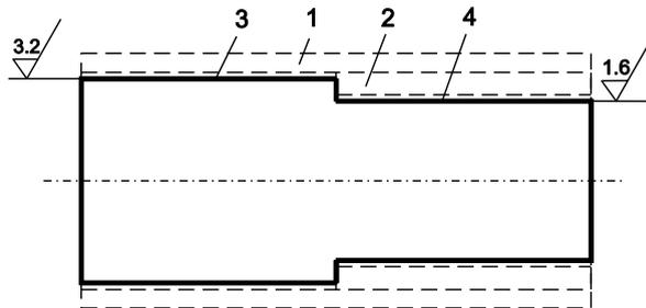
Fig. 1. Sample part cutting steps.
